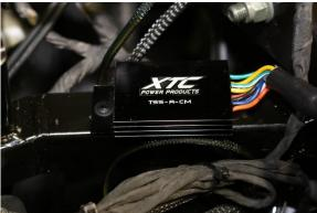
3. Plug Rear Harness into OEM Ride Command 8 pin Connector - Unplug the wire harness at the rear left side and connect our harness inline. (Note: There is a Red and Black power wire provided for an optional license plate light). The ATS-POL-RC3 fits cars with third brake light. Reach into the rear and unplug the center brake light, run the 4-pin connector to the third brake light and plug in.
