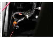
4. Run Rear Harness – Remove the seats and center plastic console. Starting at the rear run the long harness with the single 4 Pin Connector through the center of the car up the outside of the firewall through the rubber grommet to the control module and it plug in. Secure cable using the supplied cable tie's making sure to keep the harness away from any Hot or Moving parts.
