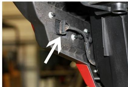
5. Drill  $\frac{3}{4}$ " holes in the front corners, remove the rubber grommet from the LED and insert into hole, push LED through grommet. **WARNING! Verify that there is clearance before drilling holes for the LED's.**
