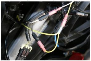
6. Test the system- and secure the harness using the included cable ties.
