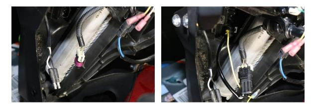
5. Plug the Turn Signal – wire into the yellow plug on the adapter. The adapter provides a secondary female bullet connector output for the original signal.
