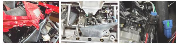
Next to the Power Steering unit is a blue connector, un-plug the blue connector from the holder by lifting on the small center tab. Plug in the adapter, attach the device to be powered, all devices installed should have there own in-line fuse The accessory port shares the same fuse as the Dash DC Outlet, it is a 10 Amp Fuse.
