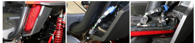
WARNING! Keep power wire away from any hot or moving parts.
