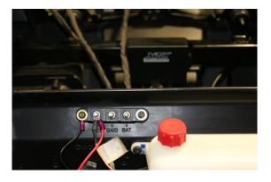
7. Verify operation of Horn. Cable tie any extra harness under dash and hood.
