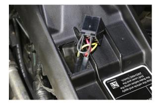
**11.** Run the power wire from the fuse block to the supplied circuit breaker, then the short end is connected to the factory busbar fulltime power (Center Stud), secure the 50 amp Circuit Breaker with the supplied screws.
