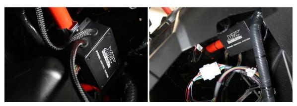
Tighten both clamps and tighten the two 10-24 mounting screws
