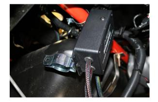
Tighten the first clamp up as much as possible before sliding the unit further over and setting the second clamp to make it easier to do the final tightening.
