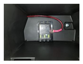
Inside Glove Box - Remove the wires from the fuse block if attached. Mount the Fuse Block inside the rear of the glove box using the #10 self-tapping screws. Drill ¾" hole in the upper left-hand corner of the box, this can be accessed from the front outside under dash cover. Install the provided ¾" grommet, insert fuse block wires into glove box and attach to terminals in the following order. Grey to fuse 1, Orange fuse 2, White Fuse 3, Red fuse 4 and Pink fuse 5.
