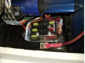
Outside Glove Box - Using the fuse block as a template mark the side of the glove box and drill with 1/4" bit.
