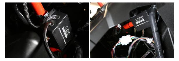
Tighten both clamps and tighten the two 10-24 mounting screws
