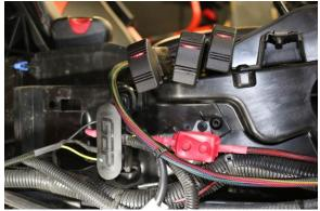
**10.** Use a cutting tool to cut out the three center console switch cutouts, trim inside of template lines and trim as needed. Mount the switches, attach the switch harness to the switches.
