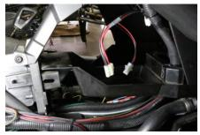
9. Plug the smaller connector into the Intercom and the larger one into the Radio connector
