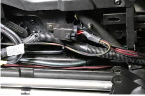
4. The Switch may be mounted in the center dash or between the seats. If up in the dash, remove the plastic panel cover in the center under the dash and run Switch Harness up to one of the factory switch spots and insert switch.
