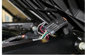
Plug the adapter into both OEM connectors as shown above.
