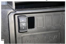
14. Run 8-pin Connector through cutout and plug switch in and insert into the opening.
