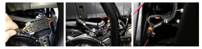
4. Run Rear Harness – Remove the seats and center plastic console. Starting at the rear run the long harness with the single 4 Pin Connector through the center of the car up the outside of the firewall through the rubber grommet to the control box and plug in. Secure cable using the supplied cable tie's making sure to keep the harness away from any Hot or Moving parts.
