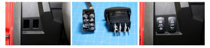
**Dielectric Grease** - LED flashers by design take very little current to activate. When water gets on the dash and lands on the top of the switch, it can trickle to the connector causing it to activate the flasher by using the switches LED indicator, the system will continue to operate and does not hurt the system but will continue clicking until the switch terminals dry. Just like the OEM we recommend using Dielectric Grease on all switch
