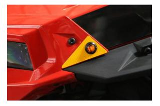
Run the short front harness through rubber grommet to the control box and plug in. Run the green wire to the right (passenger) side and connect the green wire to the black and the white to white. Run the yellow wire harness to the left (drivers) side, yellow wire attaches to black wire and the white wire goes to white. **NOTE: Black wire is positive and will not work if reversed. White is ground. Secure the Harness using the provided cable ties.**
