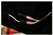
8. Lay the front small light harness out in the front under the hood, run the connector with the green wire to right side LED and run the connector with the yellow wire to the left side. Run the 4-pin connector through the hole in the fire wall to the control unit. Insert bullet connectors into LED connectors as shown above. **NOTE: The Black LED wire is positive and**
