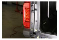
6. Secure rear wire harness making sure to keep it away from any hot or moving parts using the supplied cable ties.
