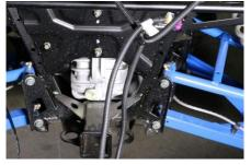
4. Unroll the long rear cable, starting with the 4-pin connector run the cable from the rear of the car over the OEM light harness connector down to the inside center tunnel and up the fire wall through the hole in the fire wall.
