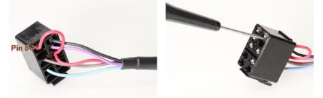
Verify operation of all lights and secure the harnesses with the provided cable ties. **Optional** - The Tan wire next to the Turn Switch is for an optional Dash Indicator. When the TSS is activated it will flash 12 VDC that can be attached to an Optional Dash Mounted LED Light.
