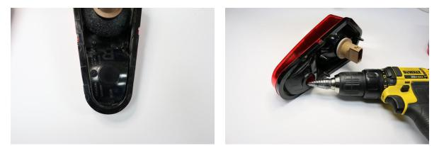
Slide rubber grommet off the LED, insert LED through the hole with wires coming out, then install rubber grommet into hole making sure wire comes through the grommet, using soapy water in the grommet, pull the LED light back through the grommet. If it seems to tight drill out holes out to 13/16".
