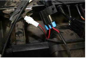
4. Run the Rear Harness - Attach the long extension harness to the previously installed rear light harness. Run the rest of the harness with the male four pin connector up to the control box and plug into the mating connector, make sure to keep the harness away from any hot or moving parts, secure with provided cable ties.
